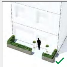
Low brick wall with an ornamental hedge
